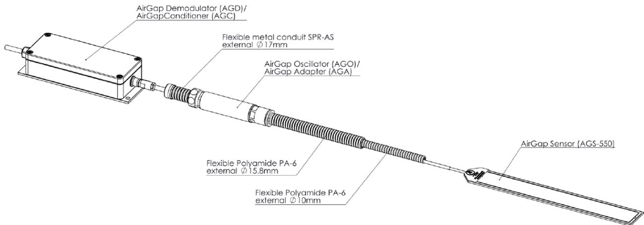
**Demodulator must be grounded!** See user manual for installation details
